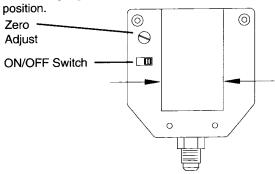
All gauges discussed here are zero adjustable. To zero the gauge, switch on and slowly turn the screw with a small screwdriver until display reads zero.
